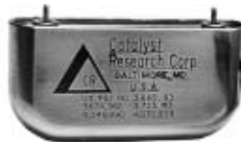
(b) Lithium-iodine pacemaker cell 2.8 V, 2.0 Ah
