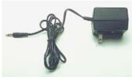
FIG. 2.32 Answering machine/phone 9-V dc supply.
