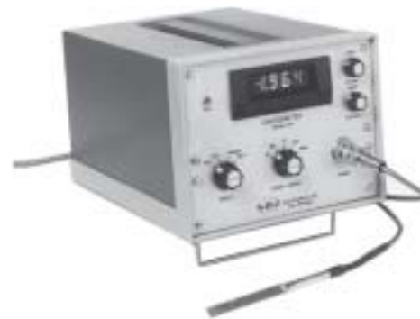
FIG. 11.16 Digital display gaussmeter. (Courtesy of LDJ Electronics, Inc.)
